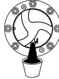
Figure 32 Draining Planetary Gear Oil
